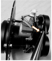
with four sensor magnets, one for each gobo slot. For showing only three gobos, remove one magnet. For two gobos, remove two magnets. Unscrew the magnet with pliers.
