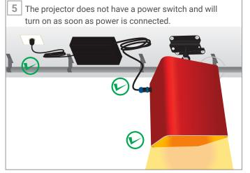
NOTE: When installing the power supply, do not add cable extensions between the power supply and the light fixture. The length of cable between the power supply and fixture should be as short as possible (6 feet maximum, 3 feet or less recommended). Any extensions required to bring power to the projector should be added on the AC side of the power supply.
