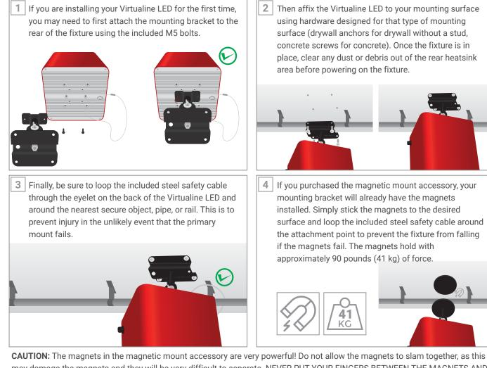
may damage the magnets and they will be very difficult to separate. NEVER PUT YOUR FINGERS BETWEEN THE MAGNETS AND THE MOUNTING SURFACE OR OTHER MAGNETS. The magnets are strong enough to cause serious injury!
